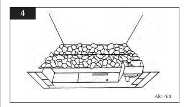
7.2 Lean the granite chippings against the burner ledges to disguise the ledges.
